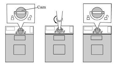
Figure 4-29 Unlocking the CPU
